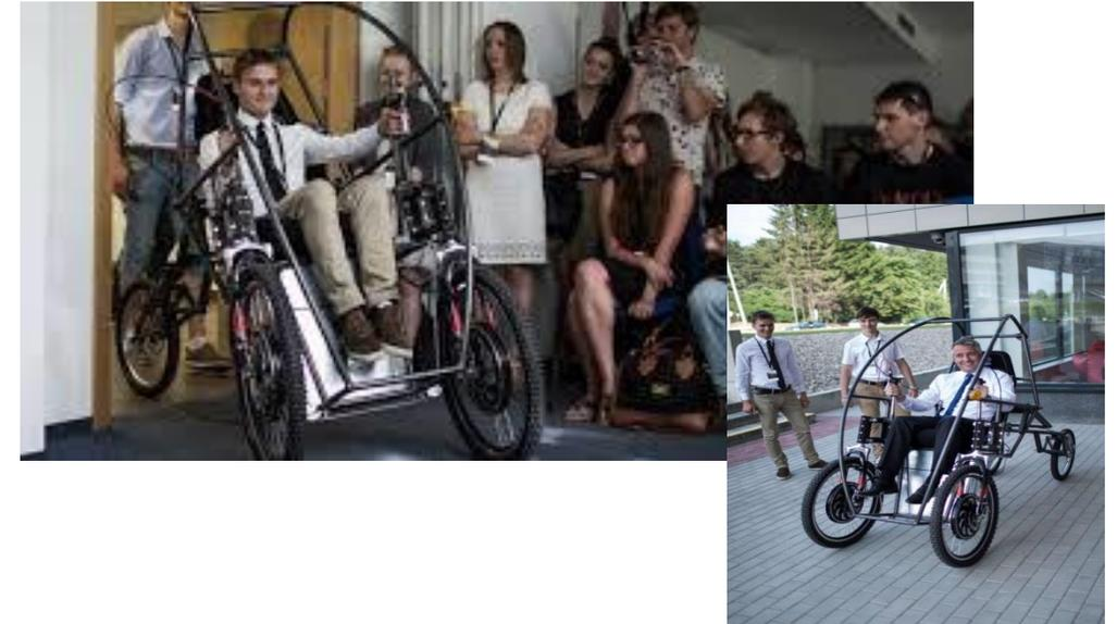
Cheap single seat electric car that fits elevator built from standard parts
